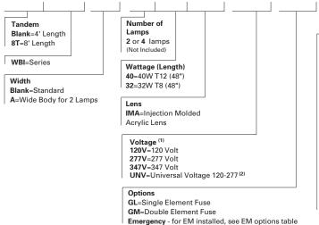
(See Options Section) Ballast Type (1) LE3=T12 Magnetic Energy Saving EB8\_= T8 Electronic Instant Start.
